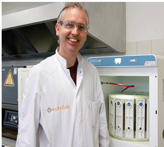
R&D manager Bart van der Nagel with Milestone's ETHOS Up microwave digestion system with which Nutrilab performs the digestion of samples for ICP-OES element analysis and ICP-MS contaminant analysis.
