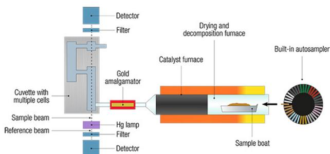
Figure 2 An Internal Schematic of Milestone's DMA-80 *evo*.
