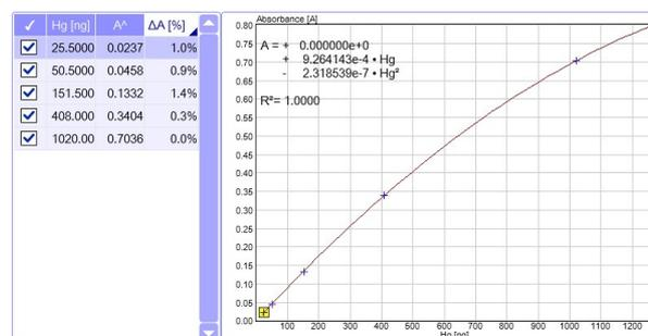
Figure 4 - 20ng – 1000 ng Calibration Graph for low to mid level
