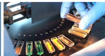
is subsequently heated and releases all trapped mercury to the double beam, fixed wavelength atomic absorption spectrophotometer. Absorbance is measured at 253.7 nm as a function of mercury content.
