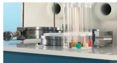
MS equipped with He and H<sub>2</sub> collision reaction cells, ultra-high matrix introduction system (UHMI) and SPS 4 autosampler. Together with our Milestone UltraWAVE and traceCLEAN acid steam cleaning system, we have the capability to tackle the most difficult samples while reaching detection limits in the parts per trillion (ppt) range.
