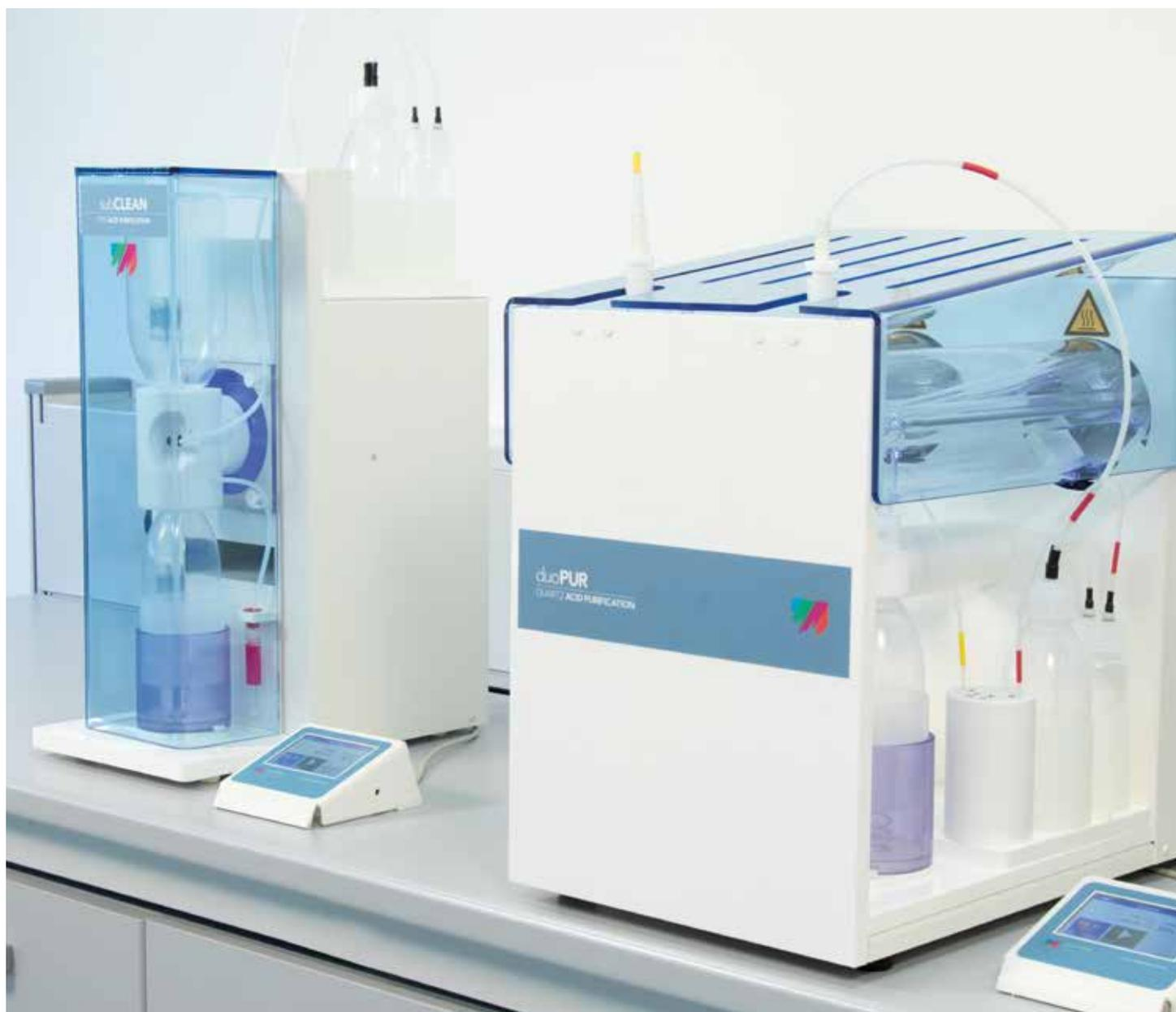
Milestone applied sub-boiling distillation technology in the duoPUR and subCLEAN. The duoPUR has two quartz purification units and allows the purification of the most common acids such as  $\text{HNO}_3$  and  $\text{HCl}$ , while the subCLEAN has a single PTFE-TFM purification still, allowing the purification of  $\text{HNO}_3$ ,  $\text{HCl}$  and  $\text{HF}$  too.
