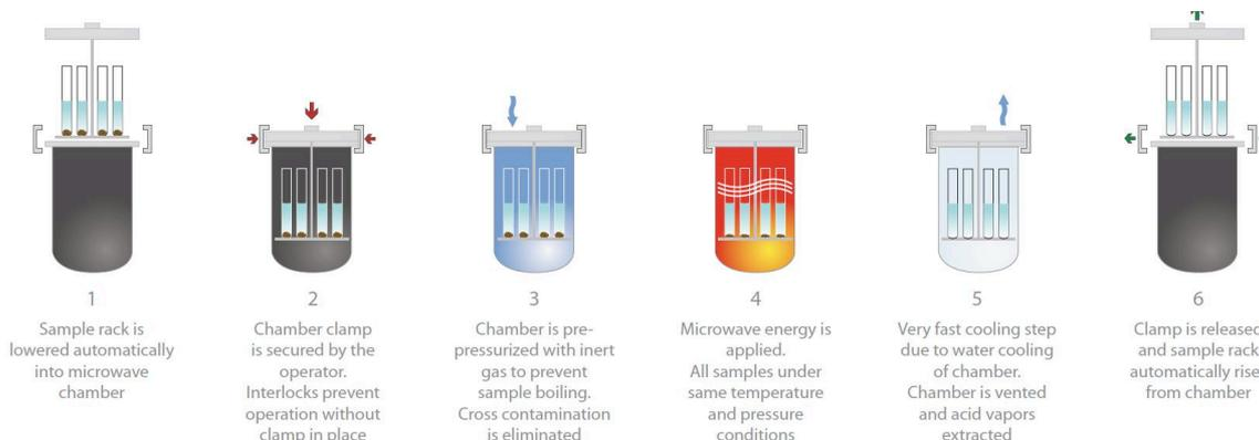
Figure 2 – Workflow of the ultraWAVE
