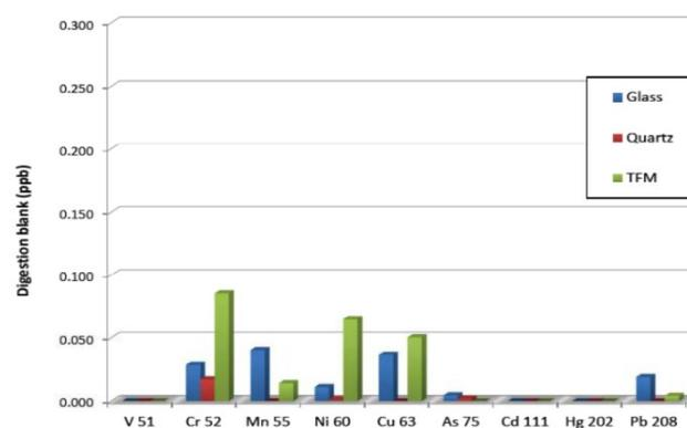
Figure 3 - Digestion blanks obtained from 2 different vial materials selected USP elements.
