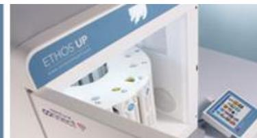
The 15-position rotor is controlled by a contactless direct temperature sensor that controls the internal temperature of all vessels throughout the digestion cycle. This ensures complete and reproducible digestions of even the most difficult and reactive samples. The SK-15 also features Milestone’s patented “vent-and-reseal” technology for controlling the internal pressure of each vessel.
